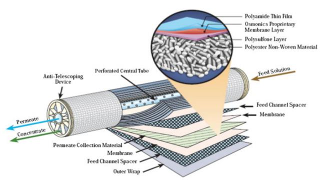
The nanofiltration membrane is composed of many different layers of thin hair-like fibers. There are different parts to the membrane such as the Permatee Collection Material and the various layers to that.
